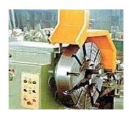
Safe Equipment – Ensure guards are in place, machines are operating correctly, safety devices have not been bypassed.
