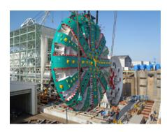
Big Bertha drilled the Seattle Tunnel; EVRAZ supplied the rebar for its reinforced concrete supporting arches.
